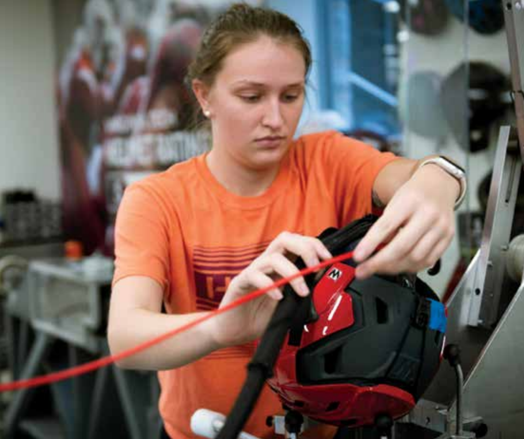
TESTING, TESTING, 1, 2, 3: Caitlyn Jung, a sophomore majoring in biomedical engineering and mechanics, sets up an impact test for a snow sports helmet in the Virginia Tech Helmet Lab. The lab's new safety ratings are the first to evaluate the helmets worn by skiers and snowboarders.
